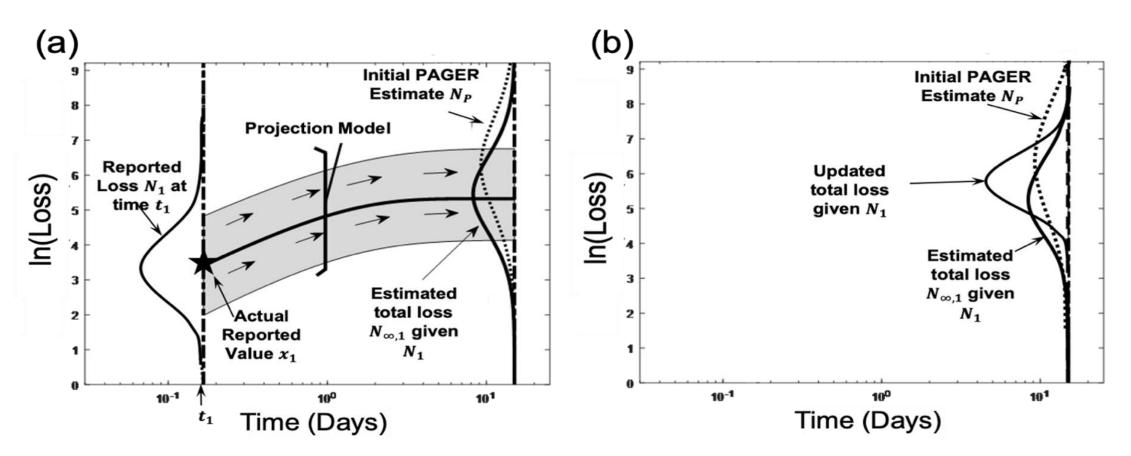
(a) The projection step, where the reported loss data at time  $\underline{t_1}$  is used to obtain an estimate of total loss based on the loss projection model. (b) The updating step, using the estimated total loss given the report at time  $\underline{t_1}$  as an observation of total loss, the PAGER loss distribution is updated to obtain a new estimate of the total loss distribution.
